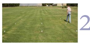
Start at the edge of the perimeter, set one rain gauge down and take 3 steps and place another cup. Repeat until you have a grid. 3. Irrigate the lawn for 20 minutes on a relatively non-windy day.
