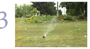
4. After irrigating for 20 minutes, combine and measure the amount of water in all of the rain gauges, divide that by 9, then multiply by 3. The answer is the average volume of water in 1 hour.
